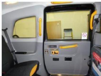
The vehicle must be fitted with yellow high visibility grab handles.
