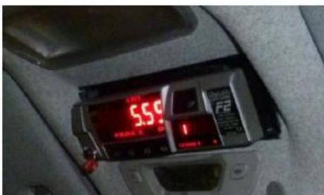
The vehicle must be fitted with a taxi meter set to the current Sandwell rates and linked to the taxi bubble light.
