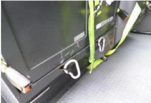
The vehicle must be fitted with appropriate wheel chair restraints.
