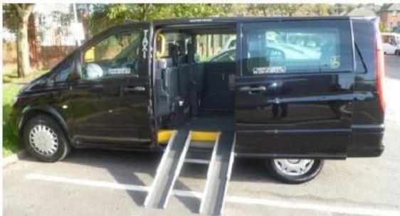
The vehicle must have side loading wheelchair access. The ramps can be detachable and stored behind the rear seats.
