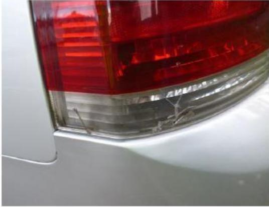
Cracked glass, lenses, lights etc. which have sharp edges or allows the ingress of water. It is not acceptable to place tape over cracks.
