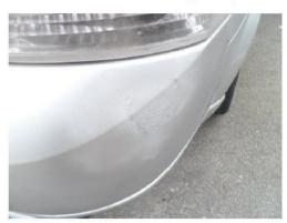
Matt paint finish is unacceptable. All damaged paintwork/bodywork must be professionally repaired and restored to the manufacturers high gloss finish.
