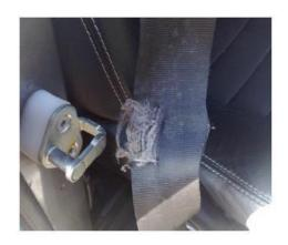
Heavily frayed or torn seat belt.
