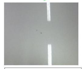
A small number of stone chips that have not penetrated the base coat of paint.
