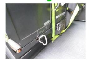
The vehicle must be fitted with appropriate wheel chair restraints.
