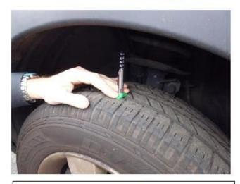
All tyres must have at least 2mm of tread across the central ¾ of the tyre. You will be advised to replace the tyre if the tread is between 2mm and 3mm.
