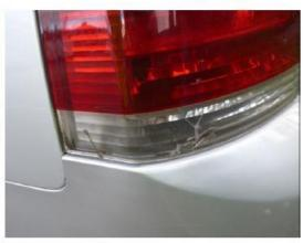
Cracked glass, lenses, lights etc. which have sharp edges or allows the ingress of water. It is not acceptable to place tape over cracks.
