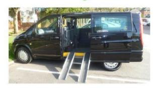
The vehicle must have side loading wheel chair access. The ramps can be detachable and stored behind the rear seats.
