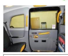
The vehicle must be fitted with yellow high visibility grab handles.
