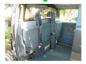
The middle row of seats must be rear facing and fold completely upright against the bulkhead to allow wheel chair access.
