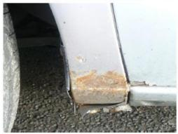
Rust or corrosion is unacceptable.
