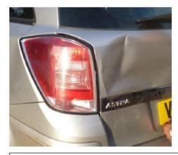
Dents that have broken the paint surface or are more than 100mm long or 10mm deep.
