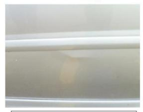
Small dents that have not broken the paintwork and are less than 100mm long or 10mm deep are acceptable.
