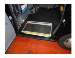
Wheelchair access may also be via a side loading integrated ramp.
