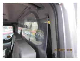
Bulkhead not sealed or in line with 'B' Pillars.
