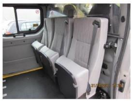
The middle row of seats does not fold completely upright against the bulkhead.
