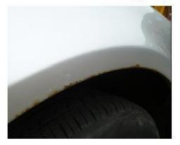
Rust or corrosion is unacceptable.
