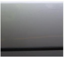
Small scratches that have not penetrated the base coat of paint.
