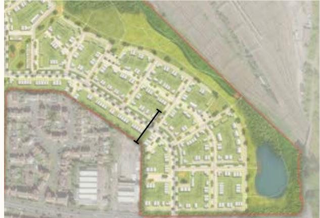
Key Plan - The boulevard has two bends along its length to force a reduction of speed and prevent rat running through neighbourhood.
