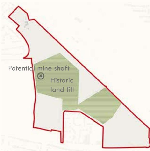
Ground conditions across the site are highly variable and are generally characterised by historical land use. The ground conditions in the central area of the site are dominated by a legacy of land-filling associated with the disposal of sewage works waste, construction and demolition arisings.
