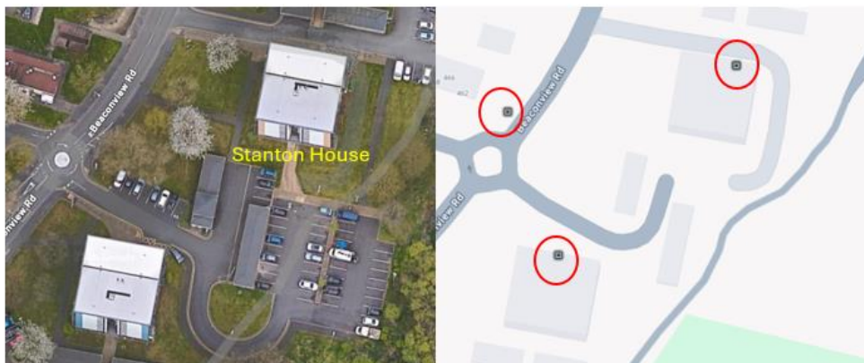
Hydrant locations marked within the red circles
